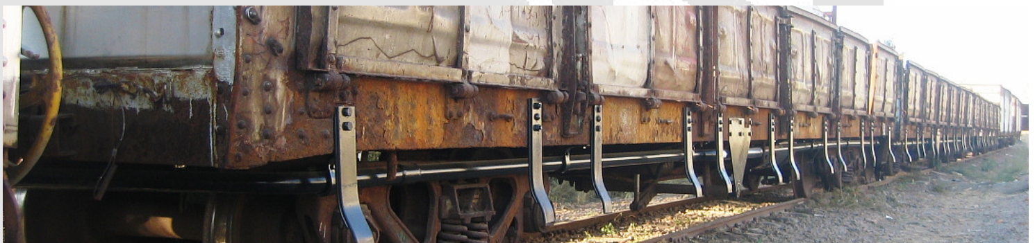
Complete new vacuum lines (including reservoirs) and door springs being fitted to Botswana Railways wagons
