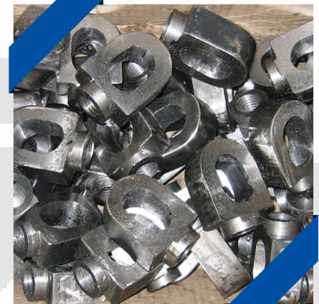
Vacuum cylinder pushrod heads
